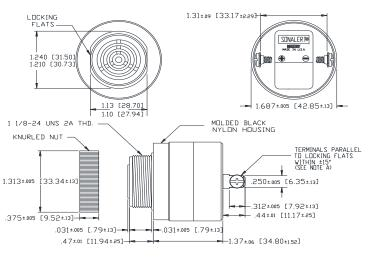
NOTE A: TERMINALS-.032 BRASS TIN PLATED, TAPPED FOR #6-32 SCREW, TWD #6-32 NICKEL PLATED BRASS SCREWS INCLUDED. WILL ACCEPT 1/4' QUICK CONNECT. NOTE B: MOUNTING- REMOVE BLACK PLASTIC NUT AND INSERT THREADED FRONT THROUGH 1.25' HOLE PUNCHED IN PANEL, IF ORIENTATION IS NEEDED, NOTE LOCKING FLATS ON DRAWING, SCREW NUT BACK ON. DO NOT OVERTIGHTEN.
