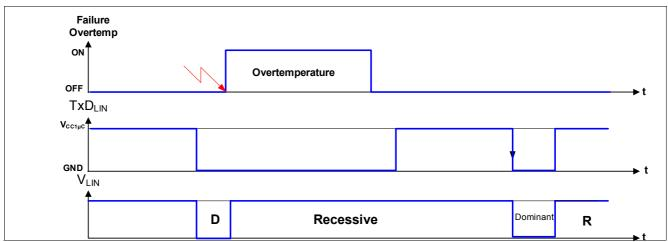
Figure 21 Release of the Transmission after Overtemperature
