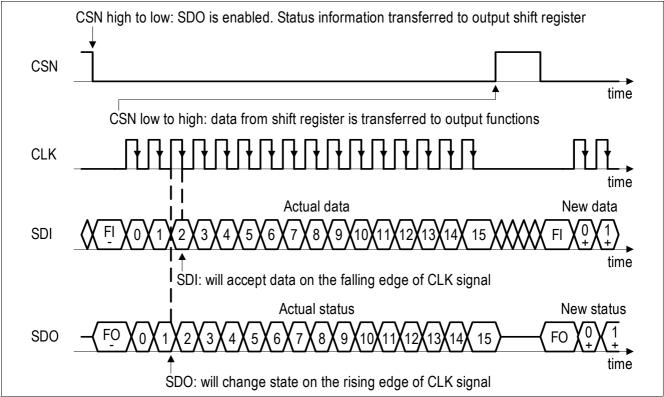
Figure 34 SPI Data Transfer Timing
