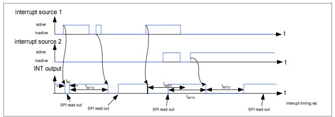
Figure 30 Interrupt Timing
