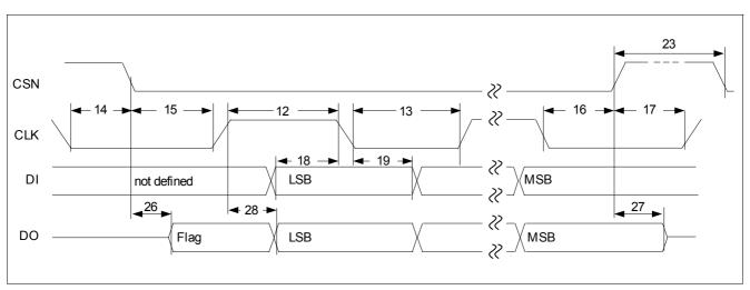
Figure 39 SPI Timing Diagram
