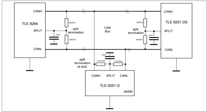
In the case the application doesn't request the SPLIT pin feature, the pin has to be left open.
