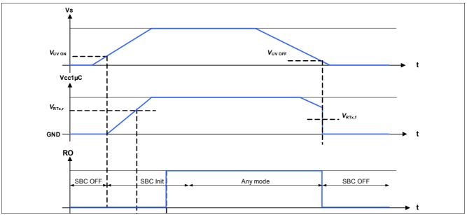
Figure 5 Ramp up / Down of Main Voltage Regulator
