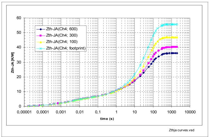
Figure 41 ZthJA Curve, Function of Cooling Area
