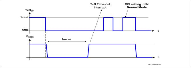
Figure 20 TxD Time-out Diagram
