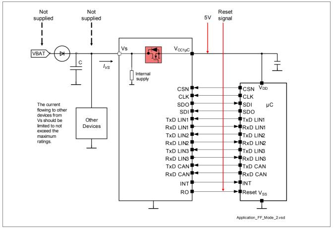
Figure 43 Application Hint for Factor Flash Mode
