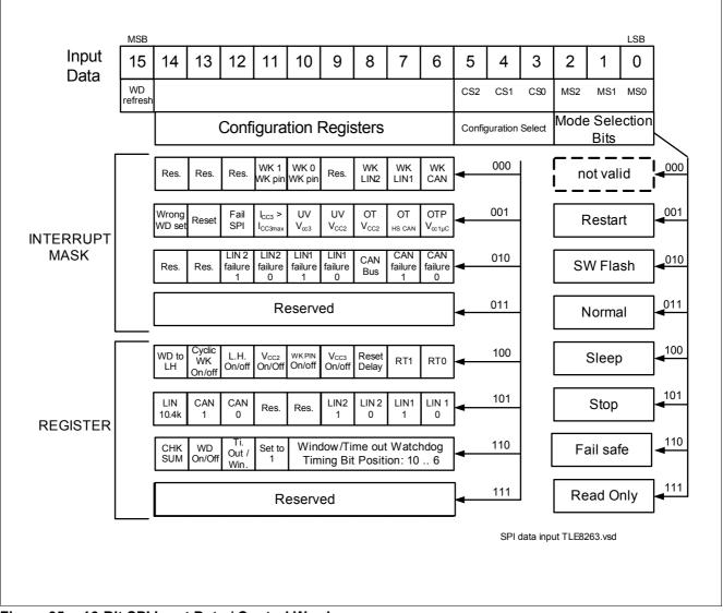
Figure 35 16-Bit SPI Input Data / Control Word
