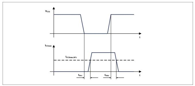
Figure 9 Regulator Reaction Time
