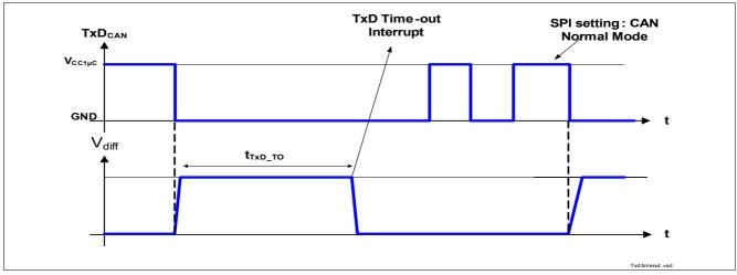
Figure 12 TxD Time-out diagram
