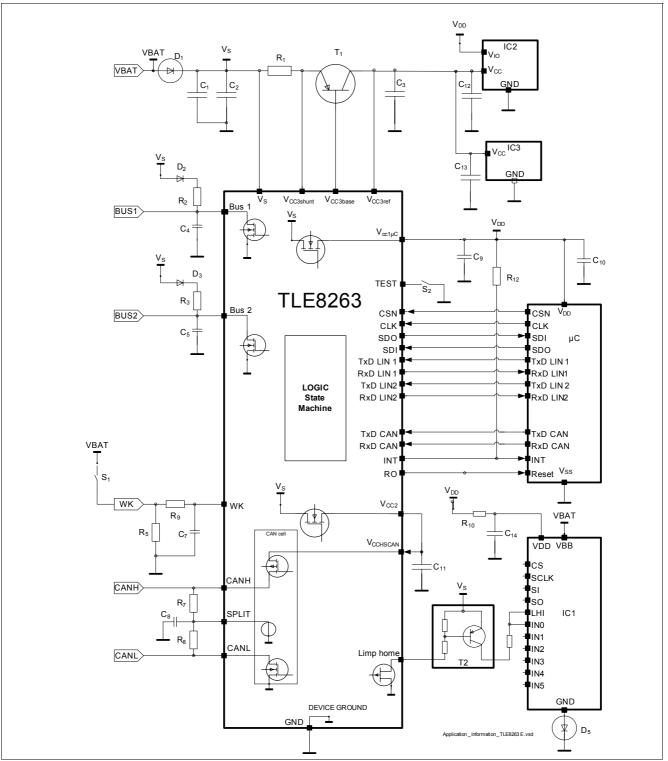
Figure 40 Application Example for a Body Controller Module
