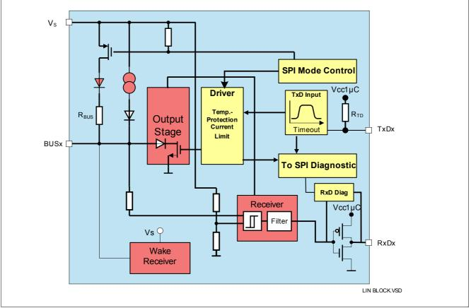
Figure 18 Functional Block Diagram
