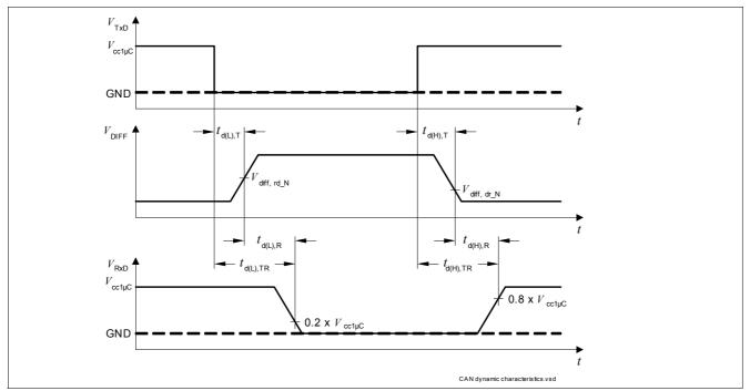
Figure 15 Timing Diagrams for Dynamic Characteristics
