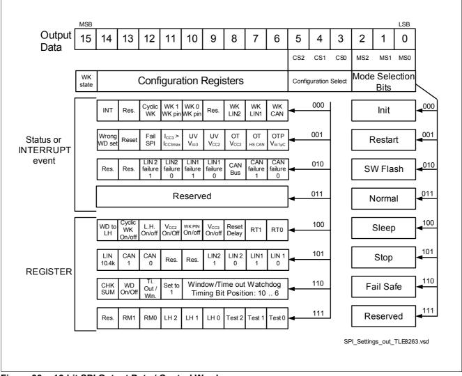
Figure 36 16-bit SPI Output Data / Control Word
