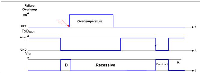
Figure 13 Release of the Transmission after Overtemperature
