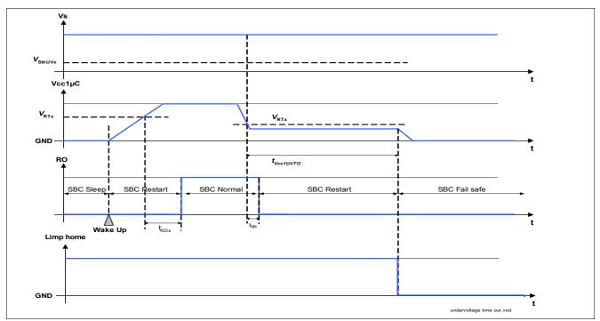
Figure 32  $V_{cc1\mu C}$  undervoltage time-out timing
