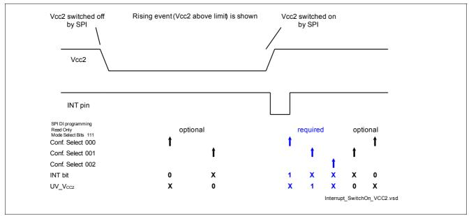
Figure 27 Interrupt Vcc2 switch-on.
