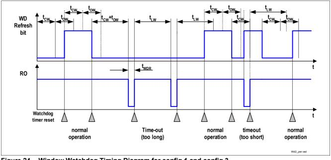
Figure 24 Window Watchdog Timing Diagram for config 1 and config 3
