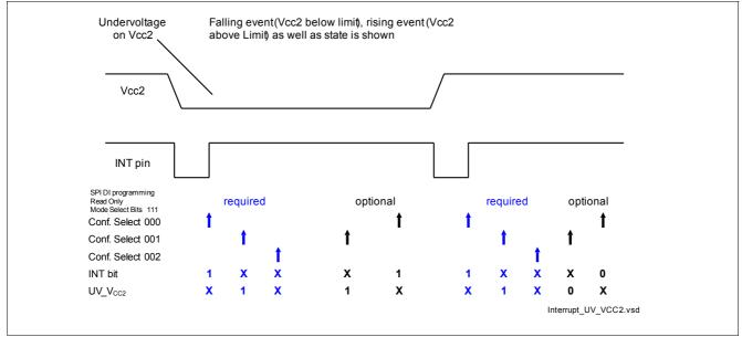
Figure 28 Interrupt V<sub>CC2</sub> under-voltage.
