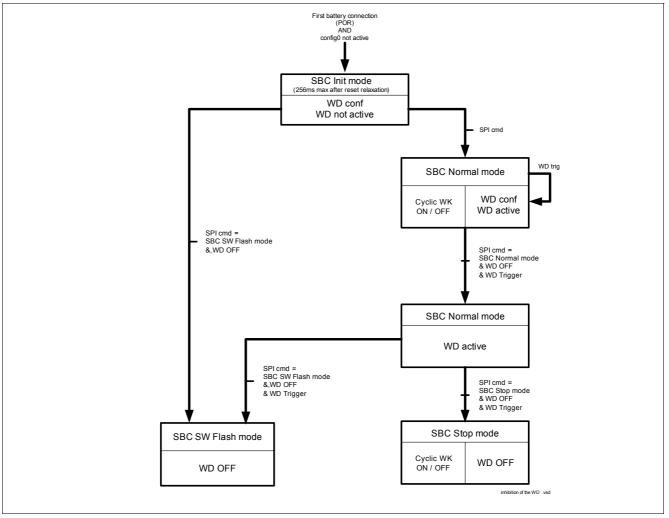
Figure 25 Inhibition of the watchdog
