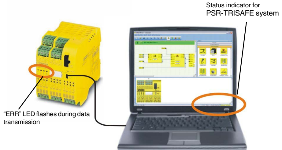
Figure 10-4 USB connection between PC and safety module
