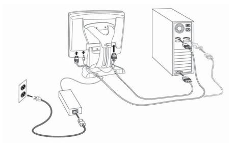
You should be sure all cable connections are secure -- tighten all cable screws. Shaking and vibration may dislodge cables that are improperly connected.
