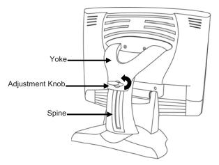
The M1500SS Display features an innovative design adjustable to approximately 60° off the vertical to accommodate different counter and user heights, a positive locking mechanism, a touch sensor interface, several mounting options, and built-in cable management.
