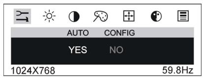
To perform an Auto Config, press the  $\triangleleft$ /left arrow key once then press SELECT. The Main Menu item Auto Config is used to adjust the configuration of the phase clock vertical and horizontal position automatically. A confirmation box is displayed to confirm the user selection. The default selection in the box is NO and is highlighted by a red bar.
