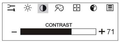
Selecting the Contrast option will allow you to adjust the contrast of the display. Adjust the contrast using the  $\triangleleft$ /left and  $\blacktriangleright$ /right arrow buttons, and press SELECT to confirm the new setting.
