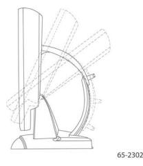
**Note:** When the adjustment knob is horizontal it is locked; when it is in the vertical position it is unlocked.
