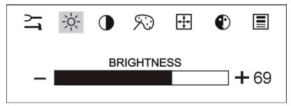
Selecting the Brightness option will allow you to adjust the brightness of the display. Adjust the brightness using the  $\blacktriangleleft$ /left and  $\blacktriangleright$ /right arrow buttons, and press SELECT to confirm the new setting.
