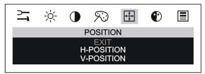
You can use the Position option to center the image on the display manually. Use the  $\checkmark$ /left and  $\triangleright$ /right arrow buttons to scroll through the position menu.
