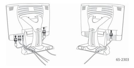
Once you have connected your M1500SS Display to your computer, you should take advantage of the cable management system designed into the base of the M1500SS Display as shown above.
